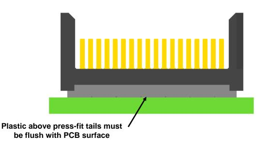
Figure 22: Proper seating depth for vertical headers
