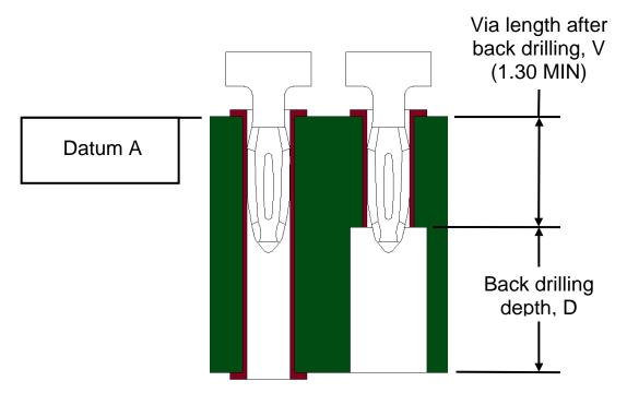
Figure 15: Back drilled via's
