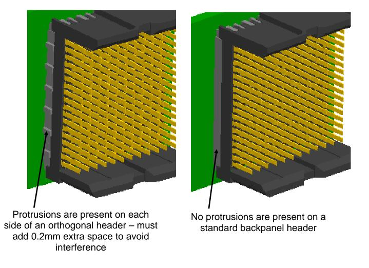
Figure 11: View of orthogonal versus standard backpanel header
