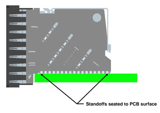
Figure 23: Proper seating depth for right angle connectors (receptacle shown)
