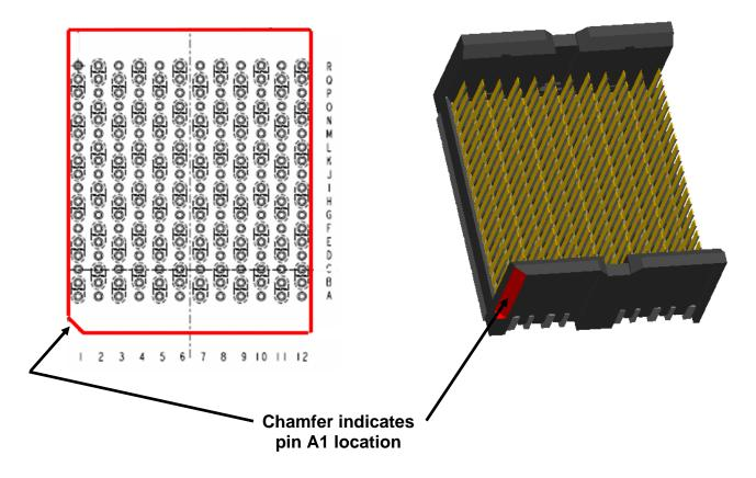
Figure 16: Vertical header outline with polarization feature
