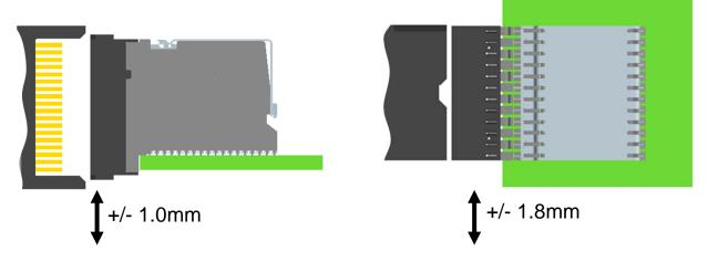
Figure 4: Connector guidance in each direction
